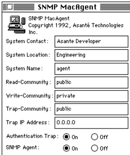
Figure 5-3 Asanté SNMP MacAgent configuration window
